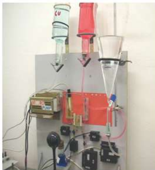
Figure 2. The photograph of the remote experiment „Galvanic cell“. Visible is the reaction chamber formed by two half cells, dividend by polymer membrane , titration pump , containers for solutions of \text{Cu}_2(\text{NO}_3)_2 , \text{C}_2(\text{NO}_3)_2 and \text{HNO}_3 acid , and for concentrated \text{Cu}_2(\text{NO}_3)_2 , and valves for letting in and letting out the solutions and acid [5]
